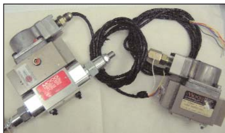
Figure 3: The CRV plate supplies a metered flow to the hydraulic valve block when it is not energized
