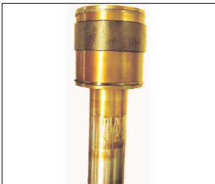
Figure 2: Varnish on the piston and rod of an IGV actuator (above) can affect turbine operation
